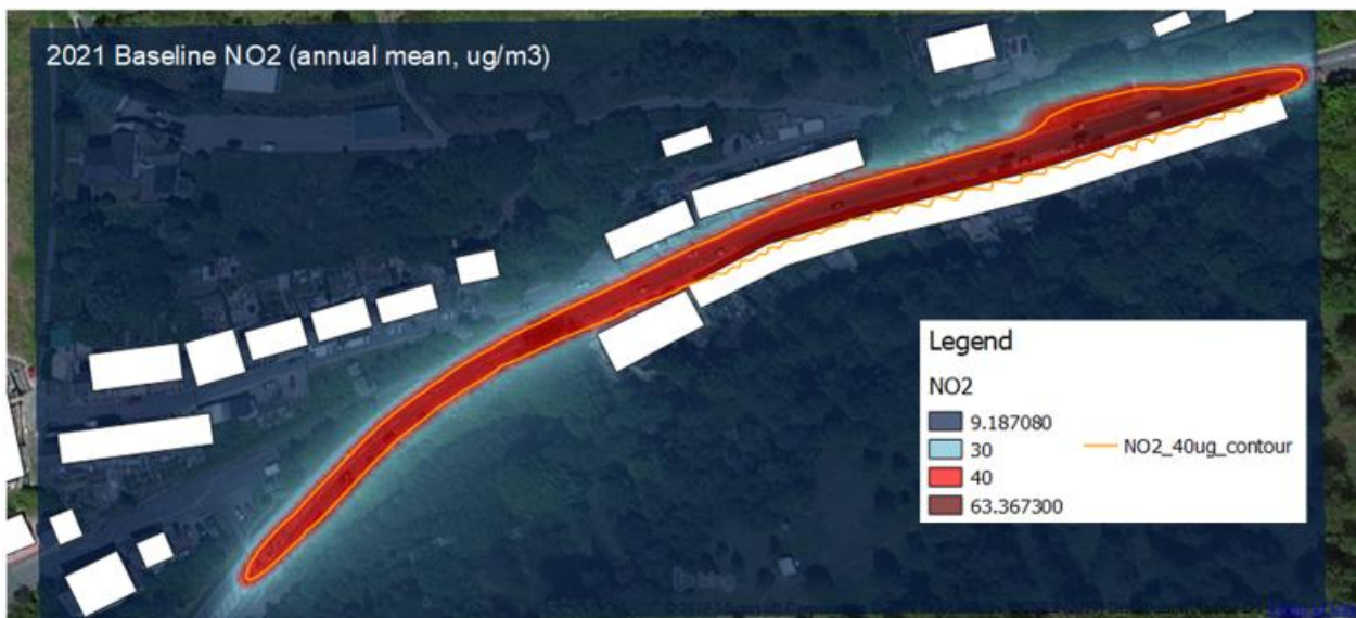
Figure 4-6 Modelled concentrations of annual mean NO 2 for 2021 do minimum
